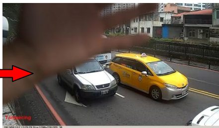
Tampering Triggered (Lens Covered)
