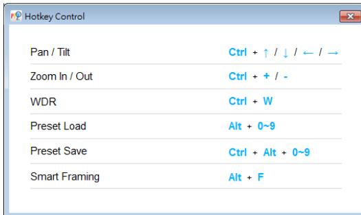
4. When hotkey control is enabled, a hotkey tip will display when mouse is moved to the PTZ control button in PTZ mode.
